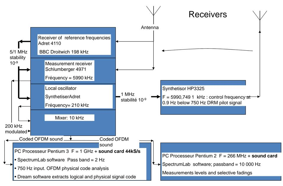
Narrow band receiver : measurement s of the DRM pilot signal disturbances (750 Hz)
