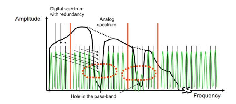
In analogic transmission; a hole in the spectrum results in a sound degradation
